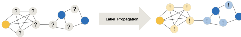
Figure 2.6.: Intuition of how in label propagation algorithms, label information flows out of the labeled nodes into unlabeled ones.
